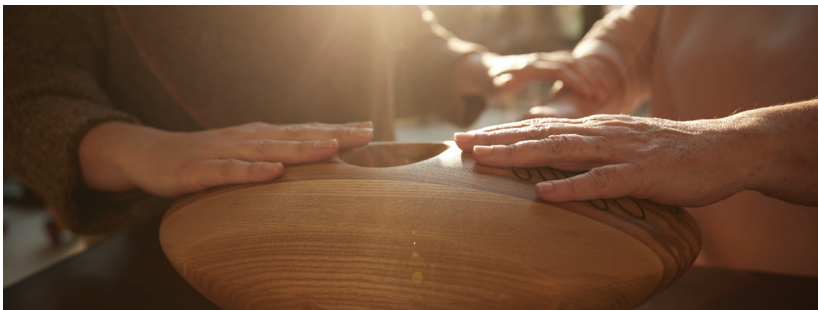
Fig. 3b: A closed circuit is being formed when users place one hand on the touchpad of the Crdl and touch each other.
